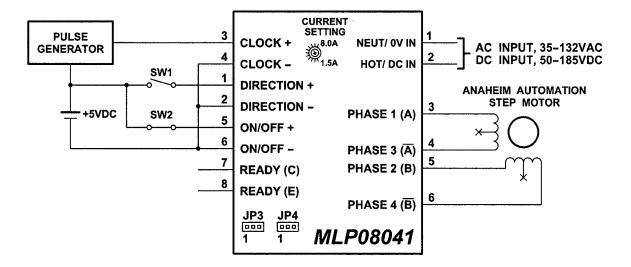
Figure 2: Hook up for current sourcing inputs
