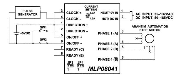
Figure 1: Hook up for current sinking inputs
