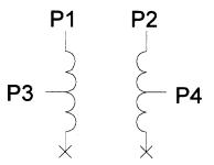
When configuring the motor in a *series configuration* (connected from end to end with the center tap floating) use the specified per Phase (or unipolar) current rating to determine the current setting potentiometer value.
